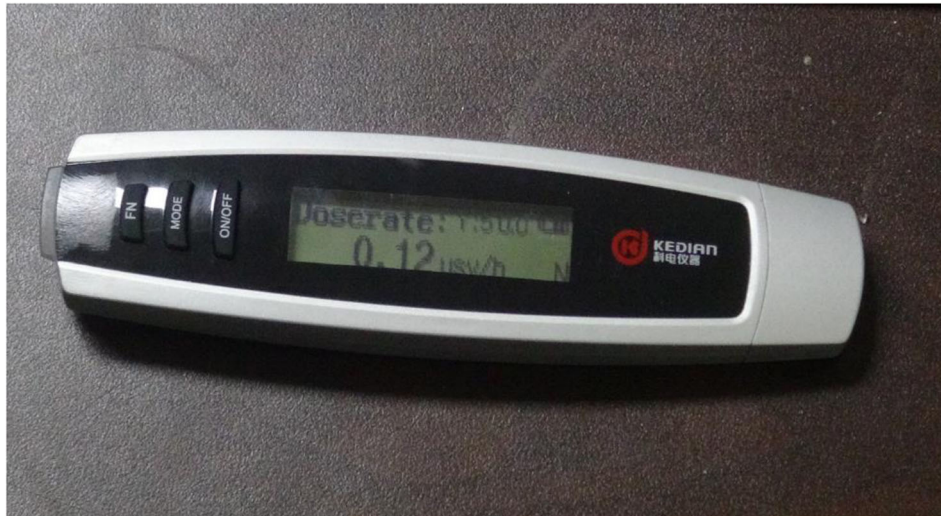
Fig. 1 X-ray dosimeter Ray 3000. It measures the radiation dose rates in millisievert per hour and microsievert per hour
