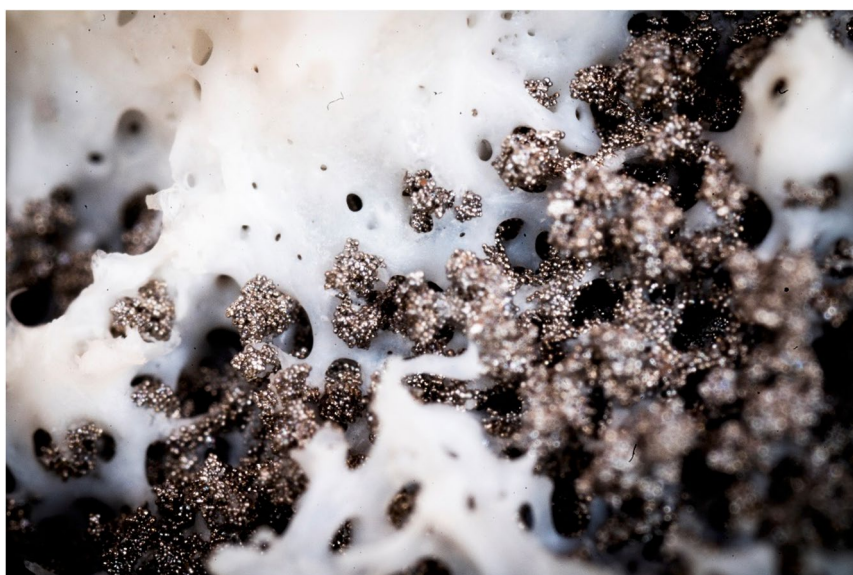
Fig. 1 Bone ingrowth into the porous coated surface of an uncemented cup (Trident® Tritanium™, revision, Acetabular System, Stryker Orthopaedics). White (bone), grey (titanium beads). Courtesy of Thor Balkhed, Linköping University
